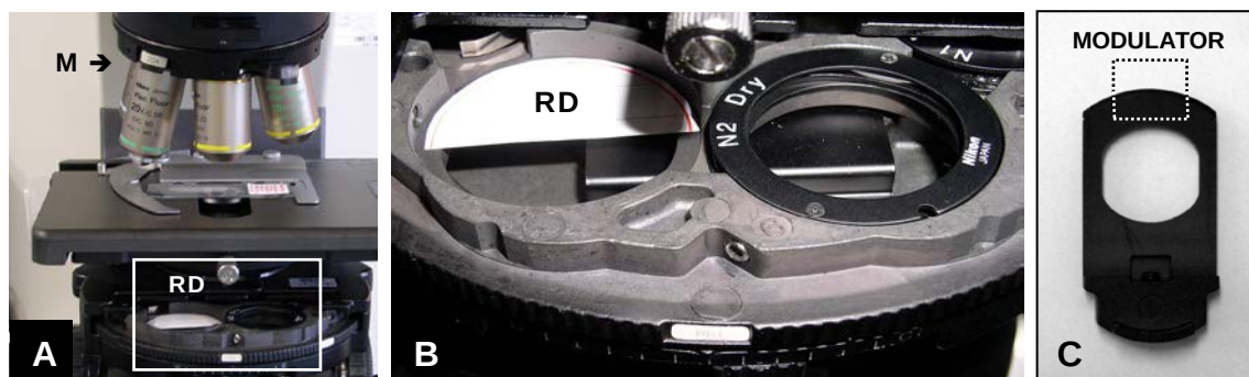
Fig. 1. Adaptation of an upright microscope to standard (RD only) and modulation (RD+M) relief-contrast imaging. Relief diaphragm (RD) is actually made of black (not white) cardboard. Modulator (M) placed in the objective back focal plane consists of an edge diaphragm (dotted square in C), much like RD.
